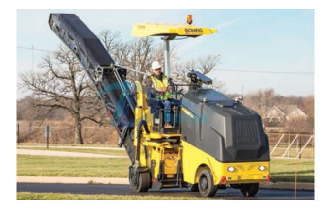
Asphalt Milling Machine
